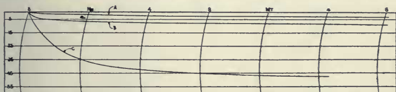
FIG. 11. Auxographic record of swelling of sections of agar 90—tyrosin 10, .15 mm. in thickness, in NaOH N/100 , A = 133 per cent., in HCl N/100 , B = 233 per cent., and in distilled water, C = 1600 per cent. \times 6 .
